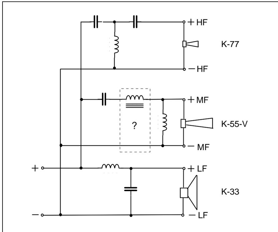
Klipsch Cornwall II crossover network (B600/6000Hz) schematic
