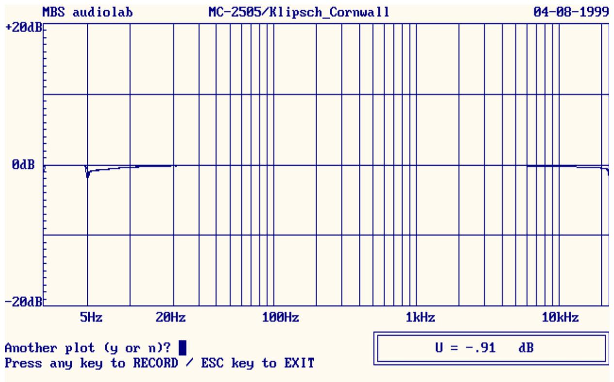
Please note, the two plots on the upper diagram obtained with McIntosh MC 2505 transistor amplifier are practically the same. The difference between them is less than 0.1 dB. Similar results could be expected with all good solid state amplifiers with higher damping factor (> 50). Please, note that amplifier frequency response is flat within 0.5 dB from 10 Hz up to 20 kHz.
