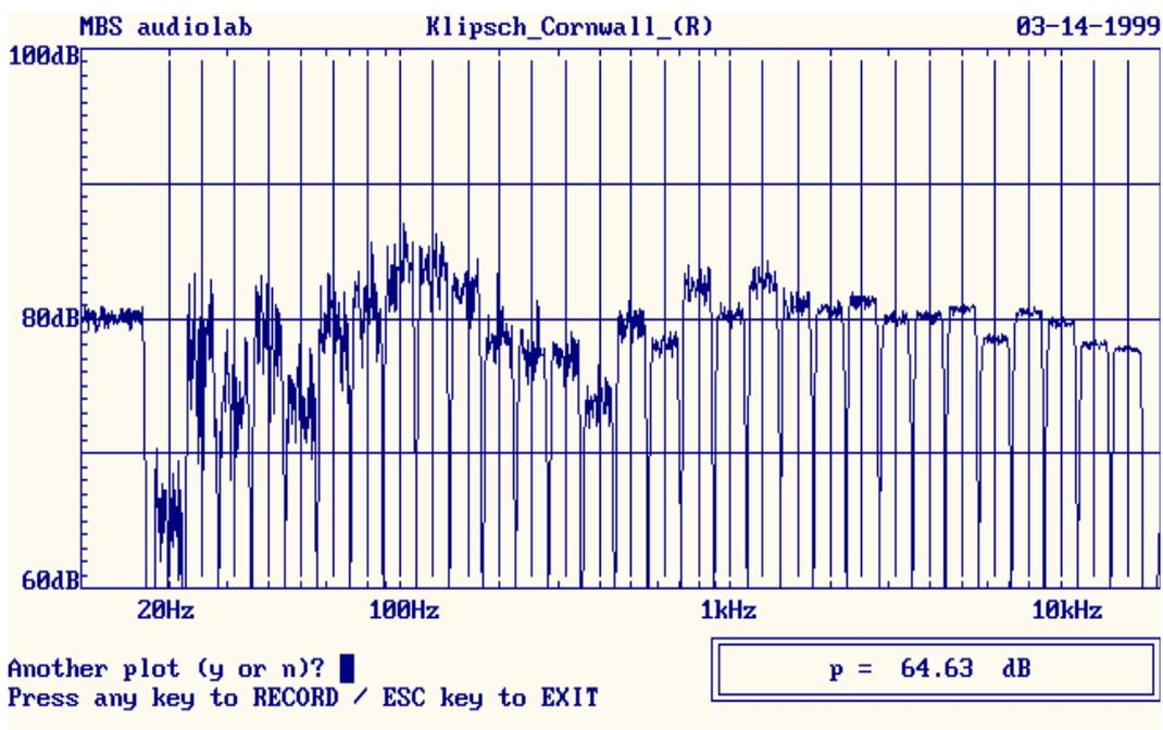
Frequency response is smooth from 25 Hz up to 20 kHz. A "deep" at 350 Hz is due to floor reflection (microphone was 1 m from front panel, and the acoustics in my quite reverberant room is not an easy problem) and a narrow resonance at 100 Hz is due to door (!) resonance.
