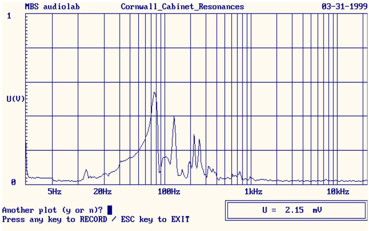
Vibrations of Klipsch Cornwall cabinet were measured in order to detect unwanted resonances, and concomitant sounds which might influence original loudspeaker's sound.
