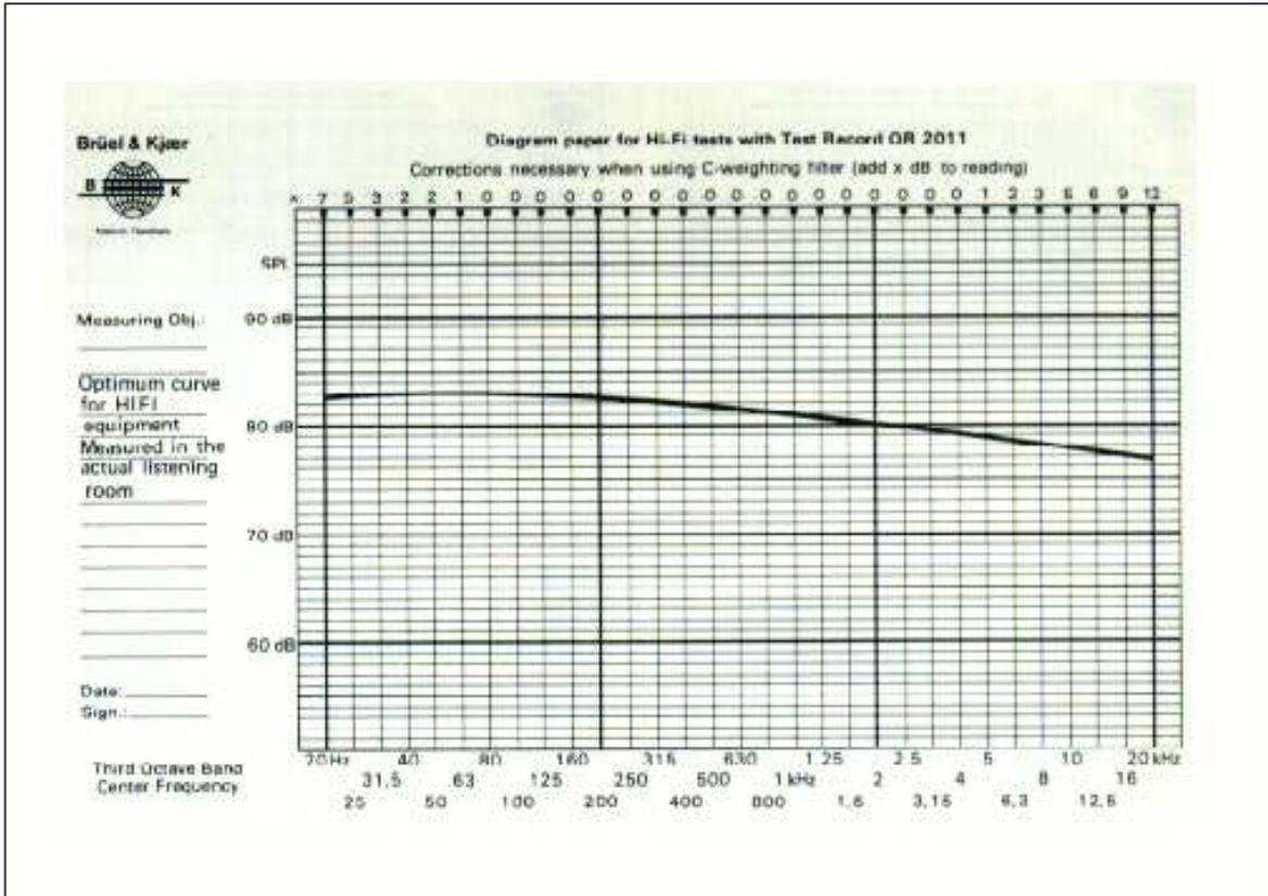
Simple explanation of this curve is that the best listening results can be expected when living room when actual frequency response of the particular loudspeaker corresponds to described curve. This curve could therefore be used as an "optimum", "calibration", "standard", "reference" or "flat" in any listening room loudspeaker evaluation.
