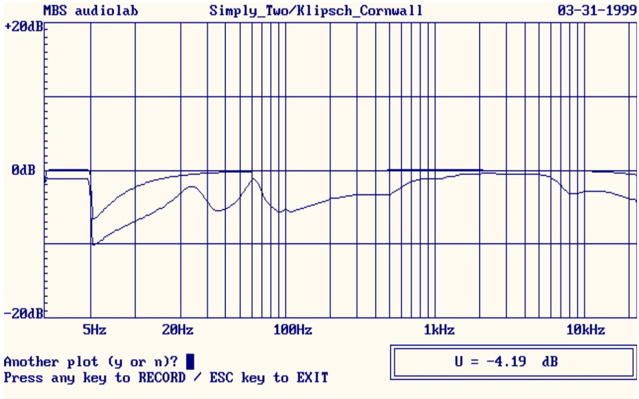
It is very easy to determine not only the differences between amplifiers, but also differences between open and closed terminals of the tube amplifier itself.
