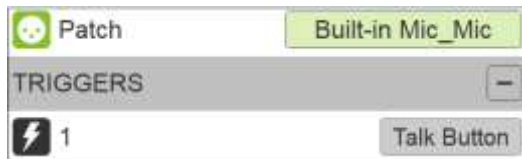
Figure 7 Example: Patching the Anubis Built-in microphone and using the Anubis Talk button as the Trigger
