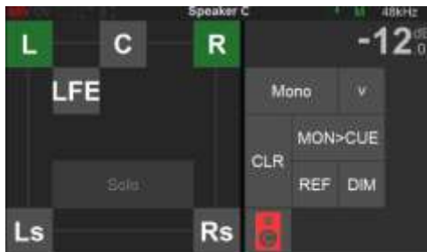
Figure 11 Example: Solo L and R channels
