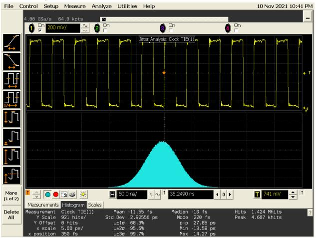
Fig11: Audio master-clock TIE analysis of the VanityPRO
