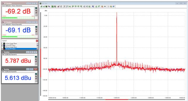
Fig1: J-test spectrum with Ligawo HDMI audio extractor
