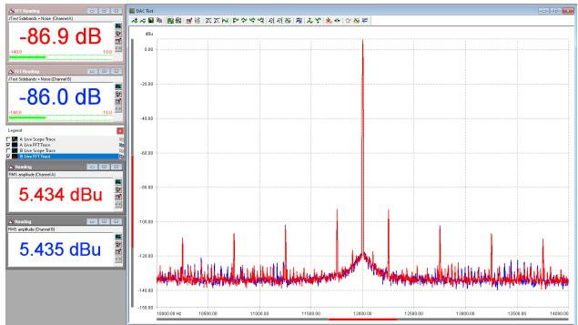
Fig4: J-test spectrum with Weiss INT204 USB audio interface
