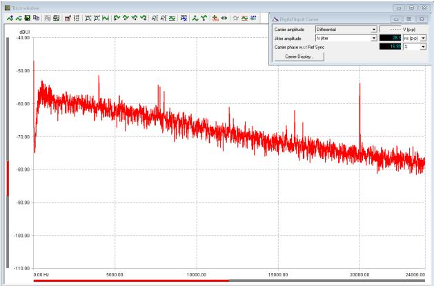
Fig5: Jitter spectrum of digital carrier with Ligawo HDMI audio extractor
