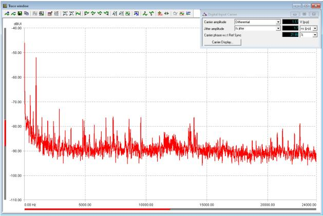
Fig6: Jitter spectrum of digital carrier with VanityPRO HDMI audio extractor
