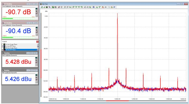
Fig2: J-test spectrum with VanityPRO HDMI audio extractor
