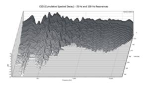
Waterfall plot of a room with a strong resonance at 100 Hz
