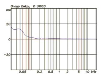
Group delay of a sealed compact three-way loudspeaker
