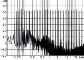
Intermodulation distortion of a two-way loudspeaker
