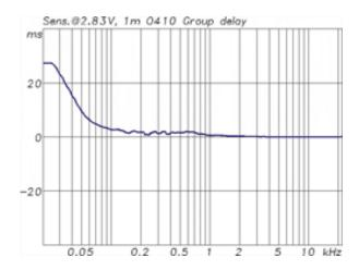
Group delay of a large three-way loudspeaker
