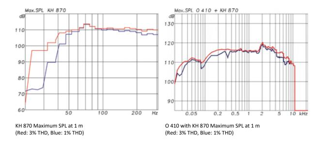
Note these measurements are for a subwoofer located in half-space. Subwoofers are typically located in quarter-space and so the subwoofer part of the curves (below about 100 Hz) would be 6dB higher.
