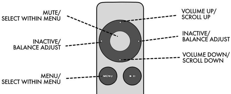
**Up and Down Buttons:** These normally function as Volume Up and Volume Down. In Menu mode, they function to move up and down in the menu as displayed on the operator display.
