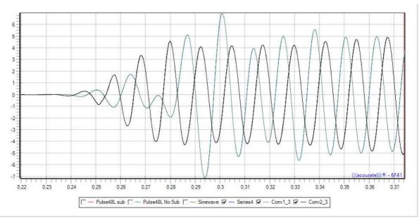
As the max peak of the main speaker is at position 12000 we add some leading zeros to the 80 Hz sinewave to see the optimal start point.
