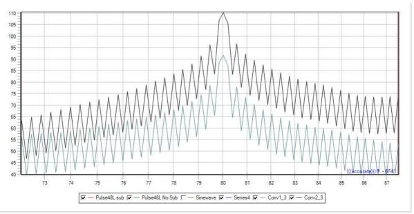
A zoom of the frequency shows that the sub signal is about -18 dB lower. So we apply a gain of 18 dB and get
