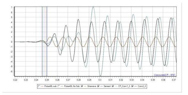
The left marker shows the positive peak of the main speakers left transition, the right marker shows the negative peak of the sub. We expect the left transition zone to be in opposite. The distance is about 225 samples. Thus the sub gets a rotation by -225 samples. This leads to a new
