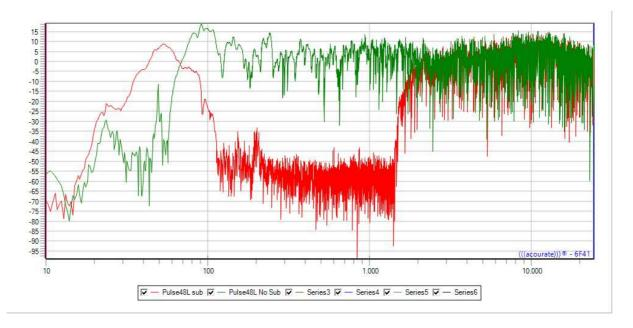
The picture shows two frequency responses. The green one is the main speaker without subwoofer. The red one is the subwoofer plus the main speaker treated by a highpass. This allows the pulse responses to be perfectly time aligned by the high frequency content in the responses. Because the high frequency content creates a peak with a high amplitude. This is demonstrated by the next picture in time domain:
