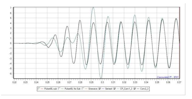
So in the steady state sub and main speakers are running together. But at the very first start we do not get the transition that we like to have.
