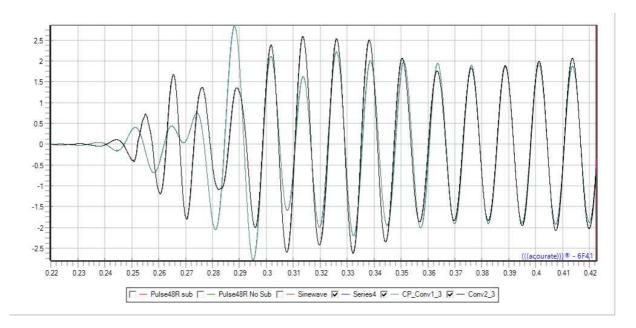
The picture shows the result with the sub polarity switched again and playing the sub 277 earlier than the main speaker.
