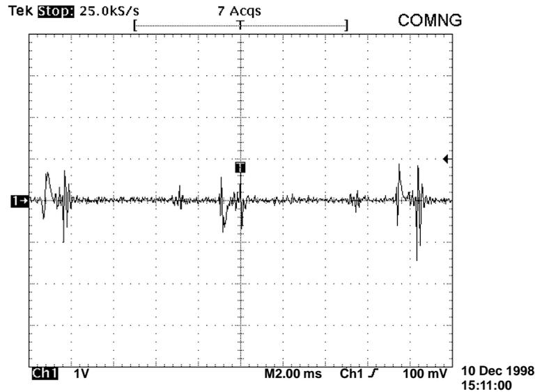
Figure 12. Common Mode Noise From Neutral to Ground
