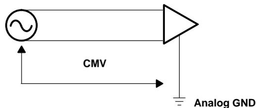
**Figure 1. Common-Mode Voltage**
