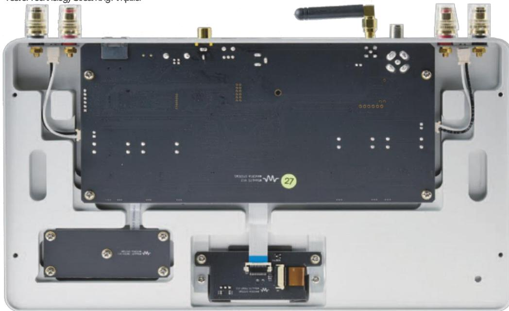
And this is exactly why the interior of the WSlim LITE appears extremely tidy. The digital output is mounted under the board and is thermally connected to the noble, solid aluminium housing. This acts as a passive heat sink.
