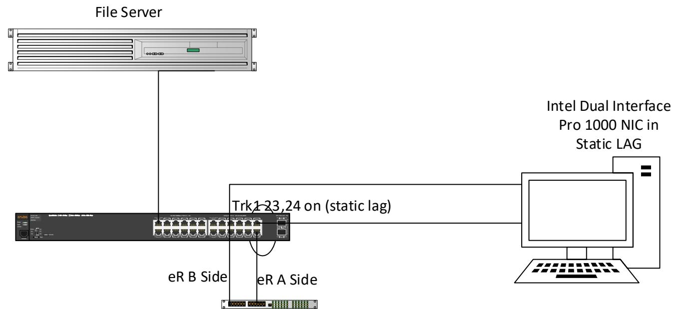
LAG goes one leg direct to computer, 2<sup>nd</sup> leg to eR A side. B side isn't in lag and goes direct to the computer.
