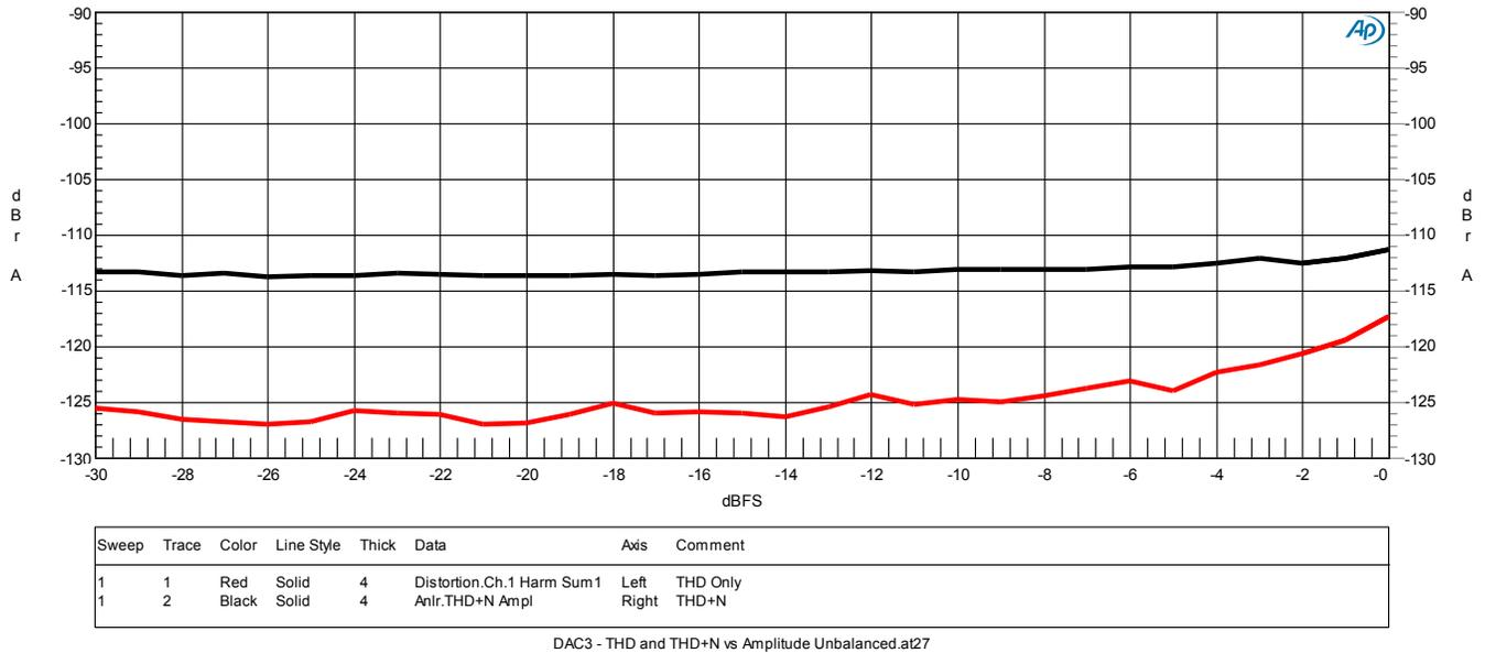
**Graph 8 - THD and THD+N vs. Amplitude (Unbalanced Outputs)**
