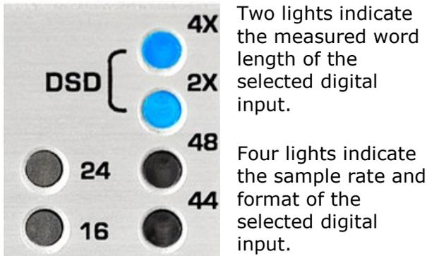
**Tip:** Computers, disk players, and streaming devices often subject the digital signal to sample rate conversion, changes in word length, PCM to DSD conversions, and other forms of digital processing that may degrade the quality of the audio. This display makes it easy to detect these processes.
