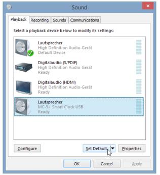
In the »Playback« tab select »MC-3+ Smart Clock USB« from the list of available devices and click at »Set Default«. after that the green check mark changes to the MC-3+USB entry.
