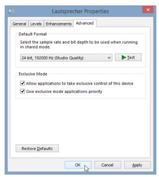
Click on the »Advanced« tab and select under »Default Format« the clock rate matching with your set-up. The optimum maner is the entry »24 Bit, 19200 Hz (Studio Quality)«. Under »Exclusive Mode« check that the two tik boxes are selected. Click »OK« to store your settings.
