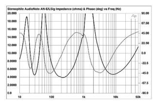
We observe that while the impedance minimum is 4 Ohm at around 220Hz, the mean impedance of the speaker is much higher. A crude analysis in excel suggests a geometric mean of 8.5 Ohm and an average of 9.5 Ohm Impedance.
