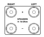
Connect the left LS3.5 loudspeaker to the LEFT SPEAKER output on the iFi RETRO Stereo 50 and vice versa.
