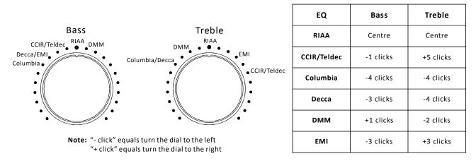
• When the mode switch is selected as Line (+6dB) input, no RIAA EQ is applied.
