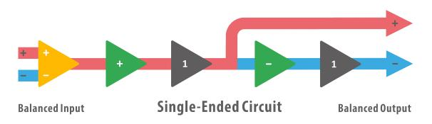
In detail: The balanced input signal will first be converted into single-ended operation by extra circuitry added to the single-ended signal path. The volume control and actual headphone amplifier are formed by a pure, single-ended circuit.
