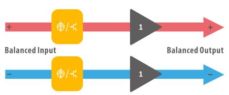
In detail: The Pro iCAN circuit is fully-balanced with completely equal circuit sections for Positive (Hot) and Negative (Cold) signal phase of each channel. The Volume control has 6-Decks, two decks each control the volume of one channel, and the other two decks are used for monitoring the volume control operation. This exceptional volume control potentiometer is custom made for iFi by ALPS Japan and has no parallel from other makers.
