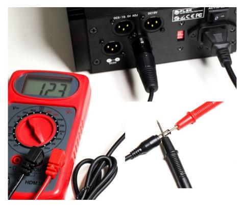
Do NOT insert the probe directly into the XLR output to measure voltage, as it might short circuit the linear power supply.
