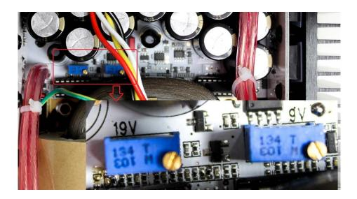
Turn the copper screw clockwise to increase the voltage, or anti-clockwise to decrease the voltage.
