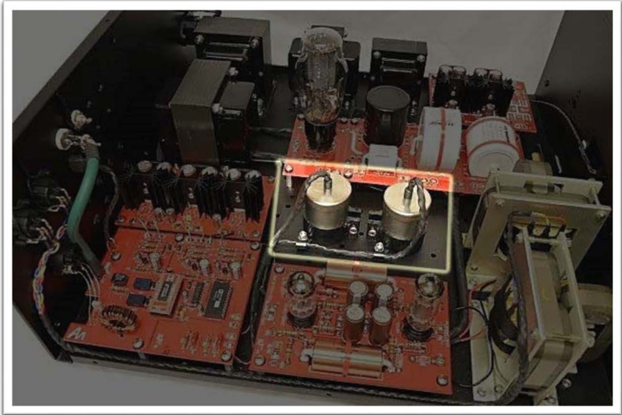
Figure 59 - Location of the I/V Transformers
