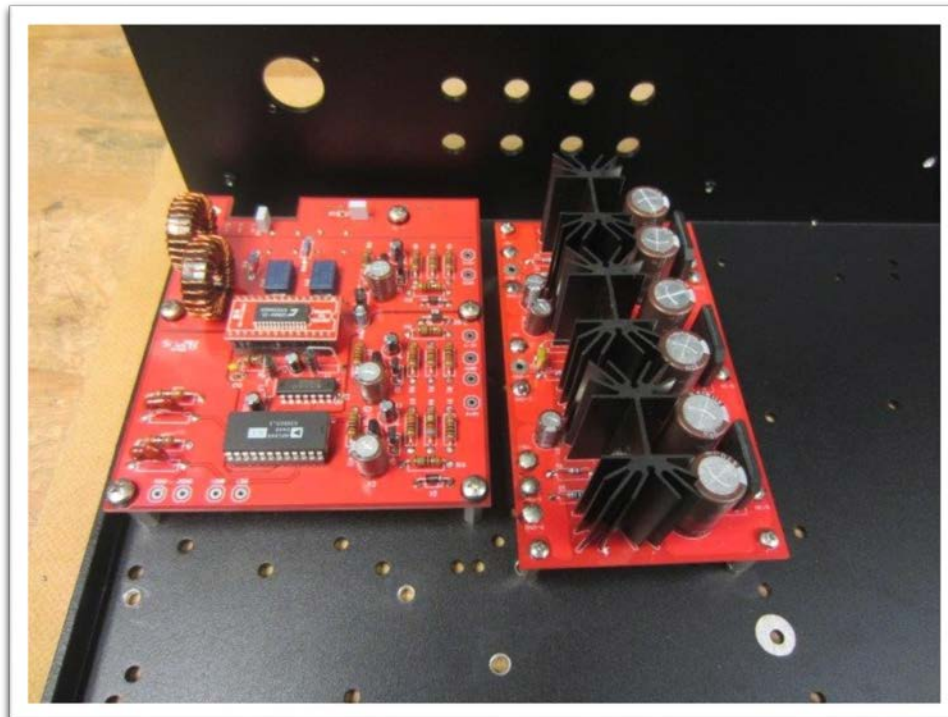
Figure 43 Digital Board installed beside the Super Regulator Board
