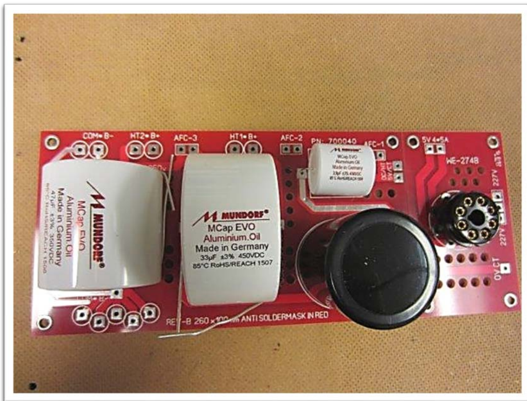
Figure 22 - Power Supply PCB and its major components
