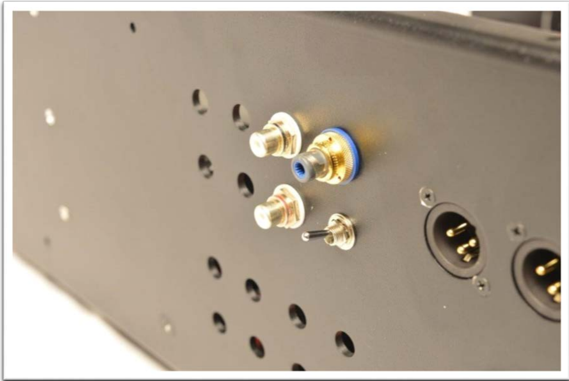
Figure 67 - Close up of the SPDIF input, selector switch and the RCA outputs from the rear of the chassis
