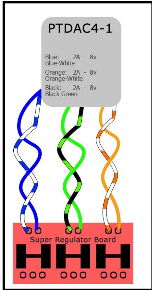
Figure 37 - Wires from the PTDAC4-1 to the Super Regulator Board
