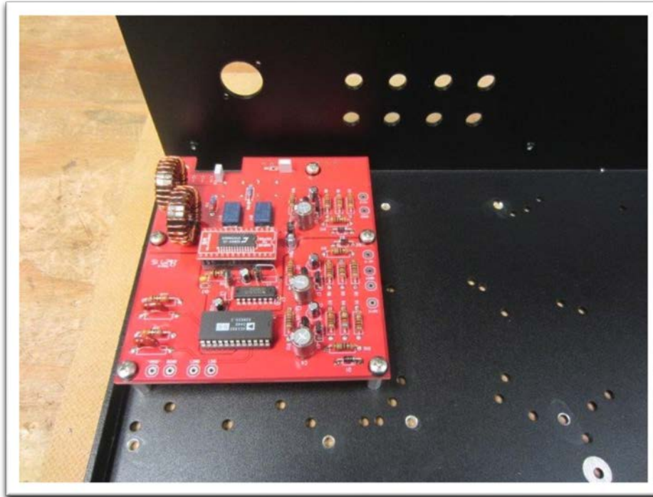
Figure 42 - Digital Board installed in the Chassis
