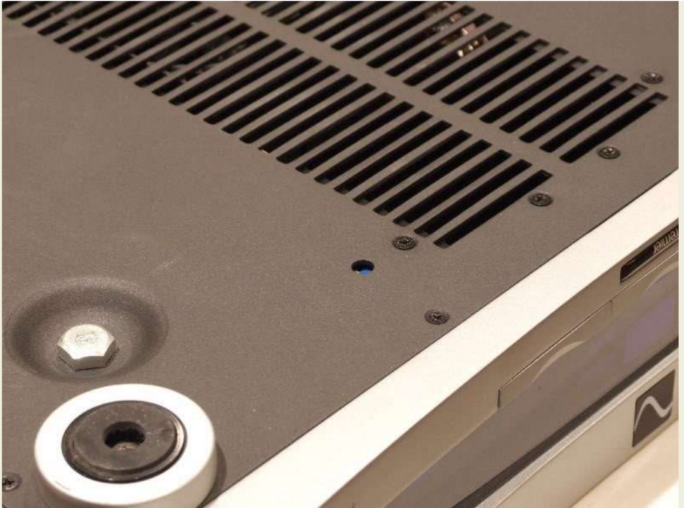
Figure 3. I see you. The "secret" trim pot for adjusting output voltage (the little blue thing).
