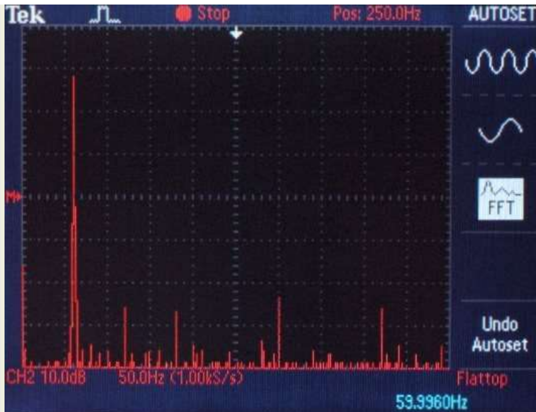
Figure 13. Power signal coming from the PPP/Premier SC power cord through the properly oriented HiFi Tuning fuse.
