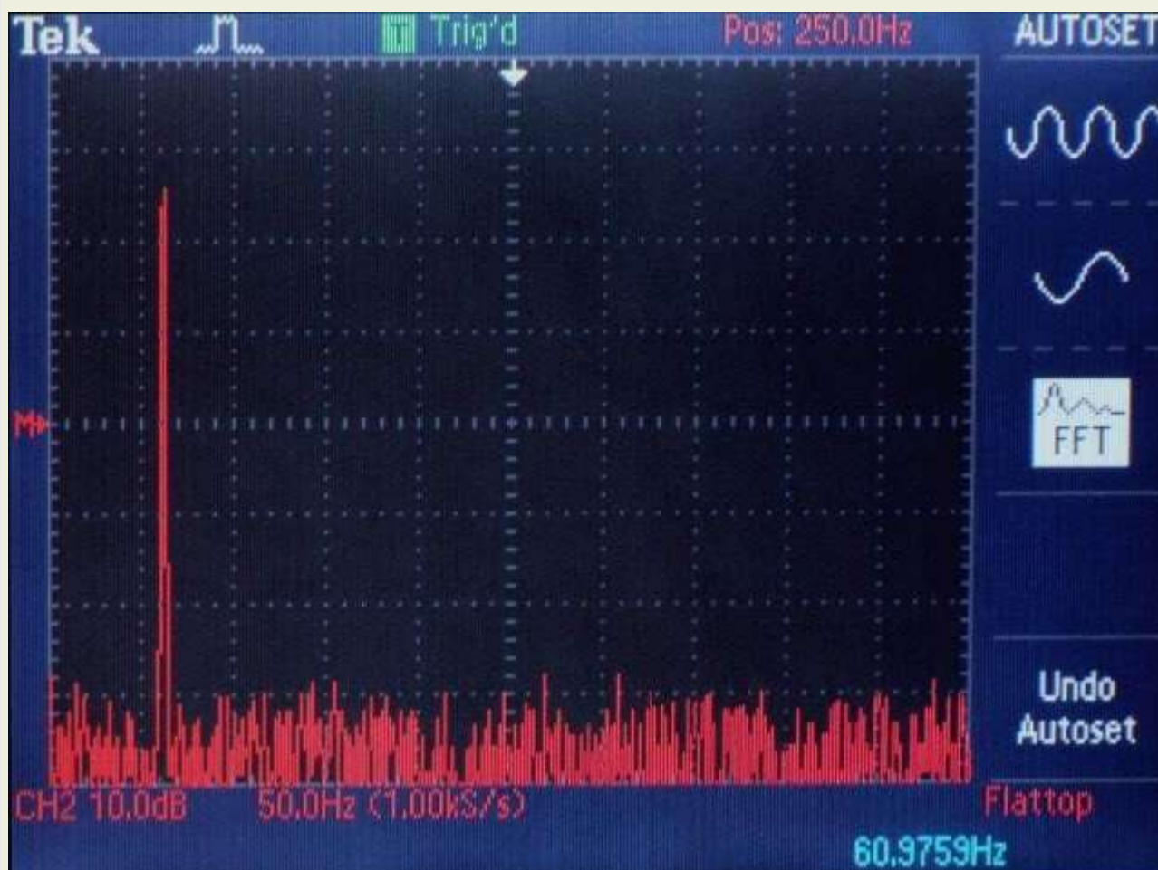
Figure 9. Dedicated audio circuit with P3 AC receptacle. FFT of 61 Hz test tone taken at right speaker SDA input.
