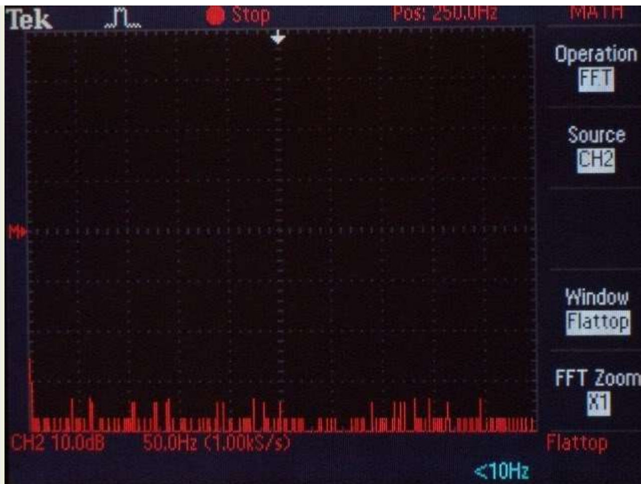
Figure 10. FFT plot of common mode noise from Soloist Premier.
