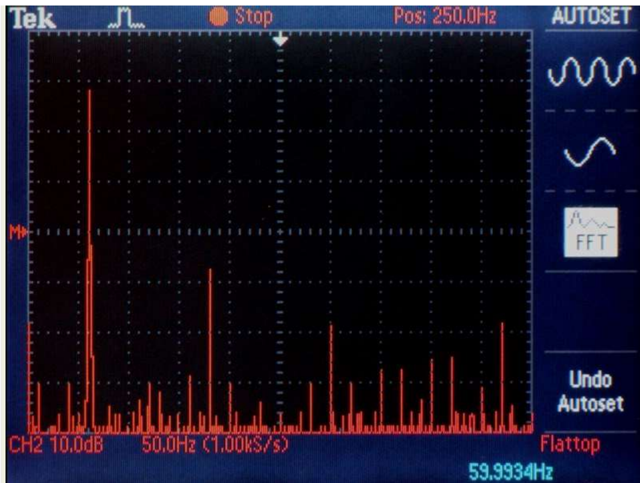
Figure 14. FFT plot from end of PerfectWave AC power cable plugged into a Soloist SE Premier in-wall conditioner on a dedicated 20 amp AC circuit.
