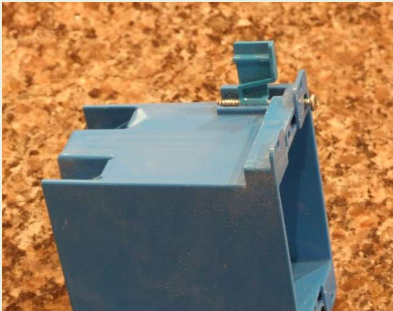
Figure 13. Aftermarket electrical wallboxes are easy to install and remove. Turning the upper and lower screws clockwise raises the retaining flanges and draws them toward the wall.
