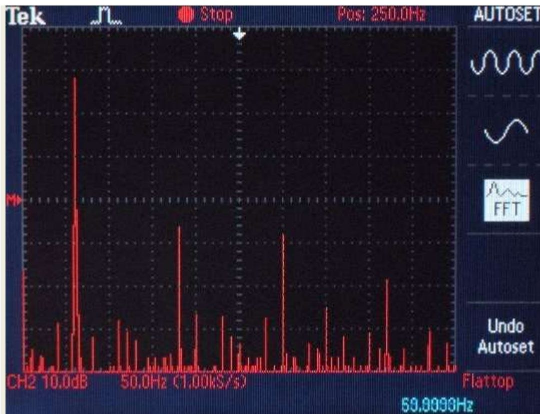
Figure 2. FFT of power signal from PS Audio Soloist in-wall passive power conditioner.
