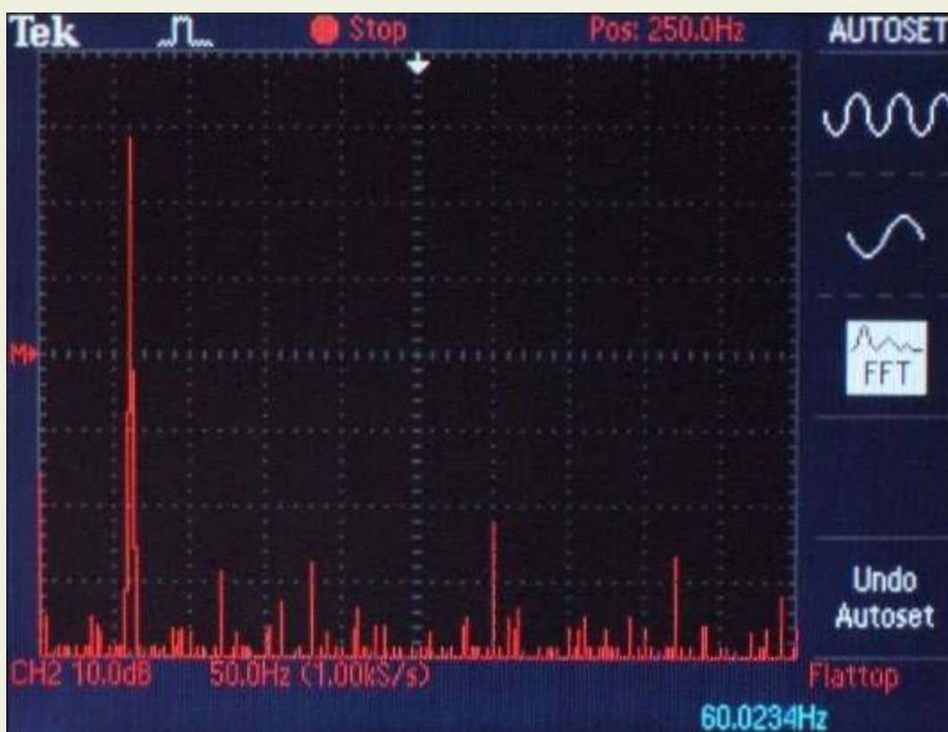
Figure 10. Power signal coming from the PPP through a Premier SC power cord. Note the dramatic reduction in harmonic and other noise compared to that seen in figures 2-9.
