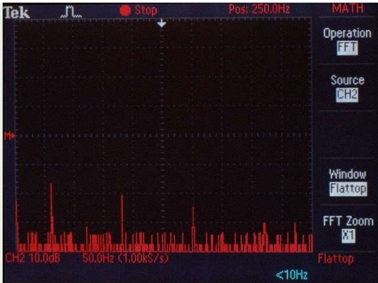
Figure 9. FFT plot of common mode noise from regular receptacle.
