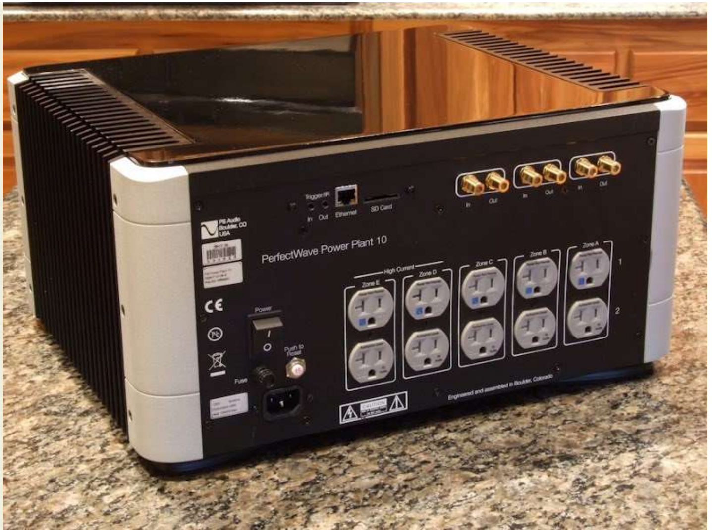
Figure 21. P10 rear. The P10 uses higher grade Power Port Premier outlets. The P5 uses Power Port outlets.
