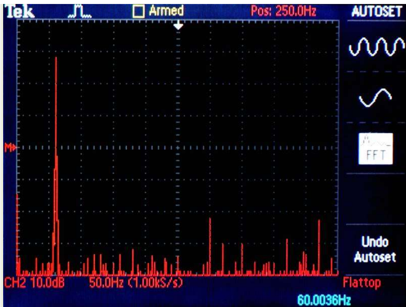
Figure 15. FFT plot from output of Power Plant Premier.
