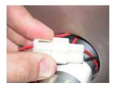
Unclip the electrical connection block and remove the whole tweeter assembly from the loudspeaker cabinet.
