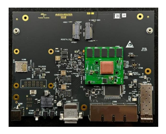
Above is a photo of the Taiko Router PCB. For comparison, below is a photo of a 3D print of the switch PCB.
