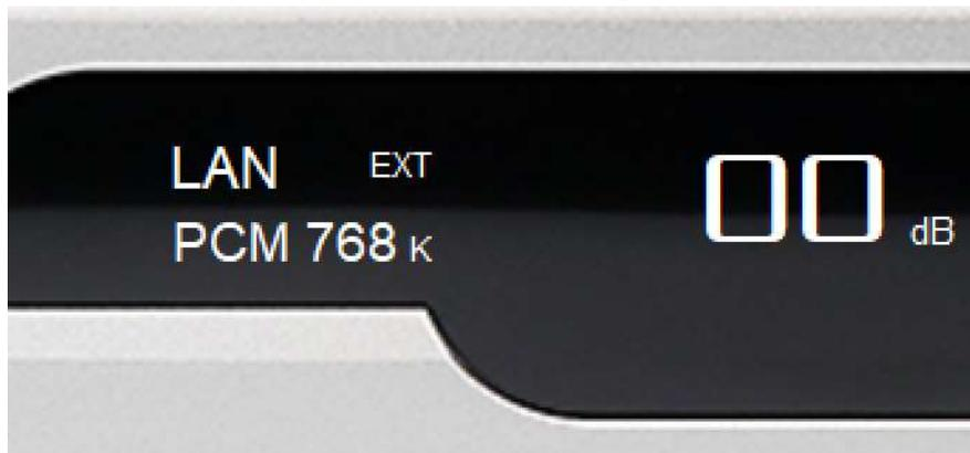
When the external clock is lost or it drifts over  $\pm 150$ ppm, the word "EXTERR" will be displayed.
