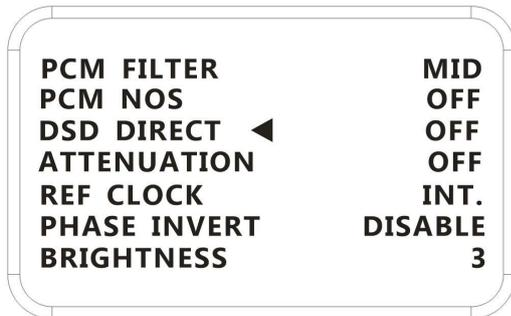
Default is OFF. Turn on to bypassing the internal interpolating FIR filter. The raw DSD stream is sent into the R-2R ladder directly.
